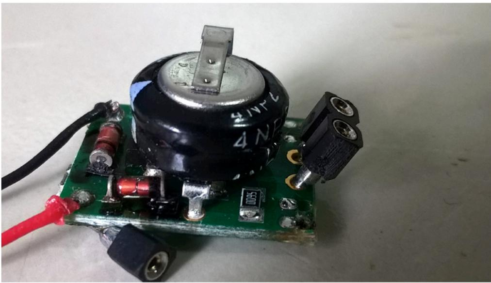
Furthermore, I would like to point out that the modern GFK/Carbon bodies are power-conducting and can cause a short circuit on the SMDs if the installation sites are not properly insulated by varnish or glue. The same applies to the included (service) exhaust sleeve. So isolate these with glue for the SMDs from the inside.
